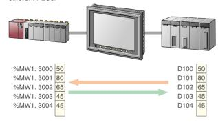
When a new facility has to be extended to an existing facility, the old facility can transfer data with the new facility's PLC via POD, without any program change of the old PLC.
