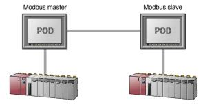
Modbus communications can be used from a personal computer to access the internal memory of POD and memories of PLCs and inverters.
